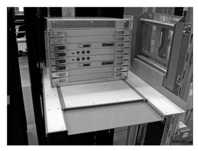
Figure 13. Chassis half way into cabinet on load plate
